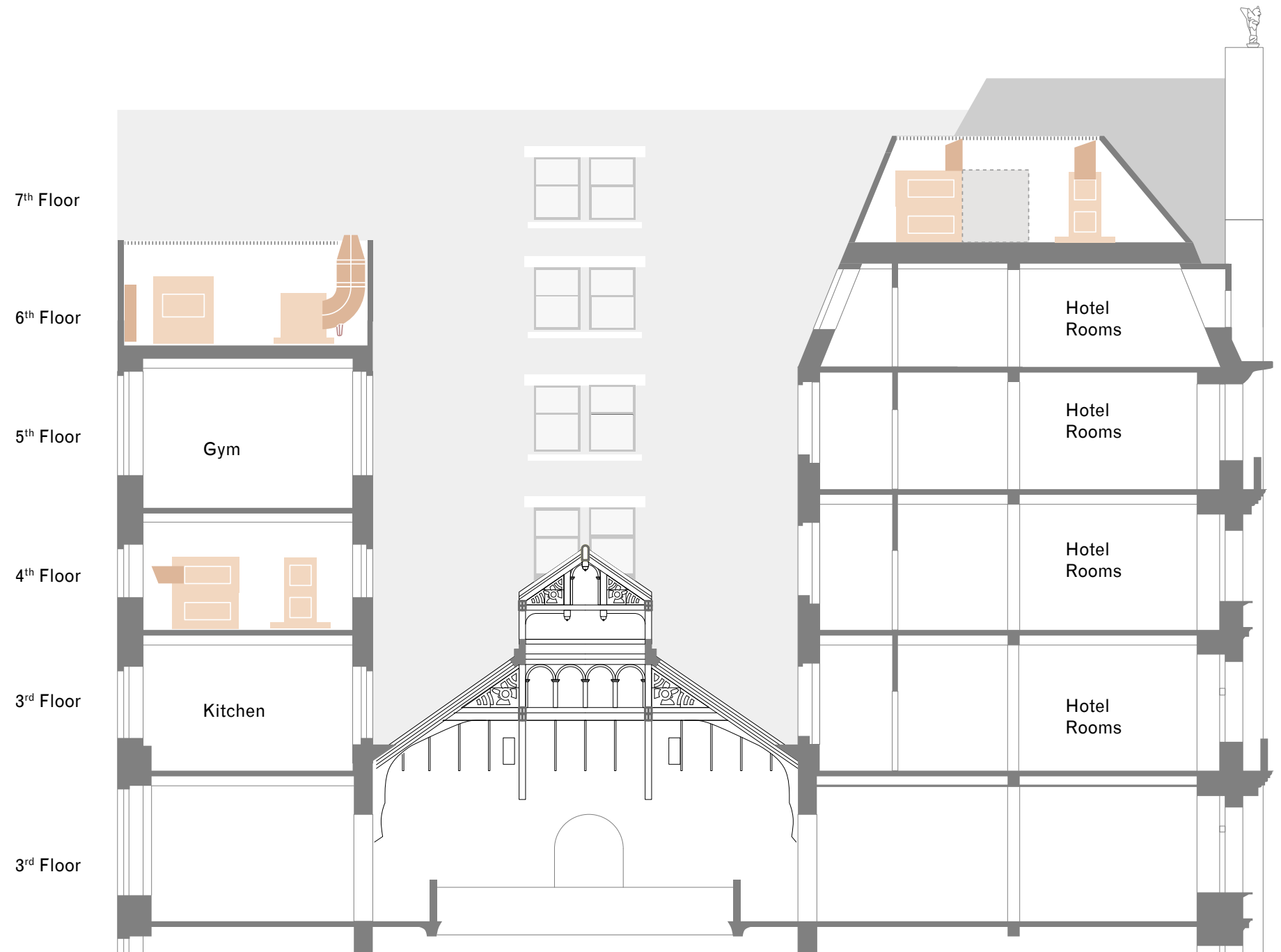
Section diagram showing the plant equipment on the roof and the mansard design
