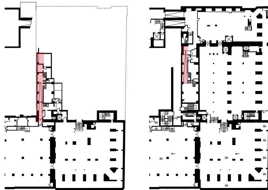
Basement levels - ramp mitigates 2.5m level difference, along a series of back of house rooms
