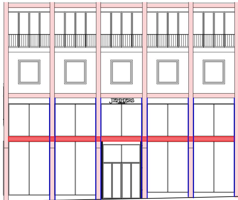
Diagram showing the beam that needs to be removed (red) and the strengthened columns (blue)
