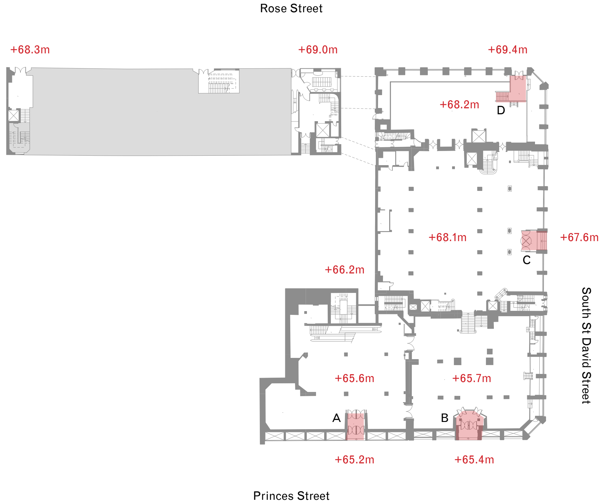
Existing ground floor levels, with main public entrances highlighted red (photographs on next page)
