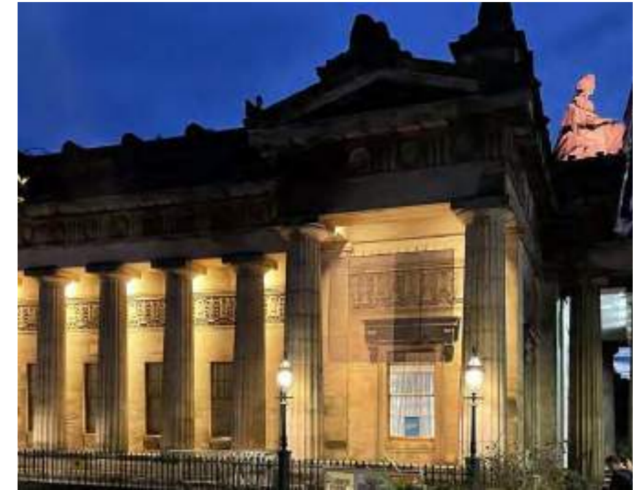
Some understated façade lighting examples can be found in nearby buildings. A good strategy is to use luminaires in a smart way, where architectural elements conceal luminaire and express the three-dimensional of the building without employing too many light sources.
