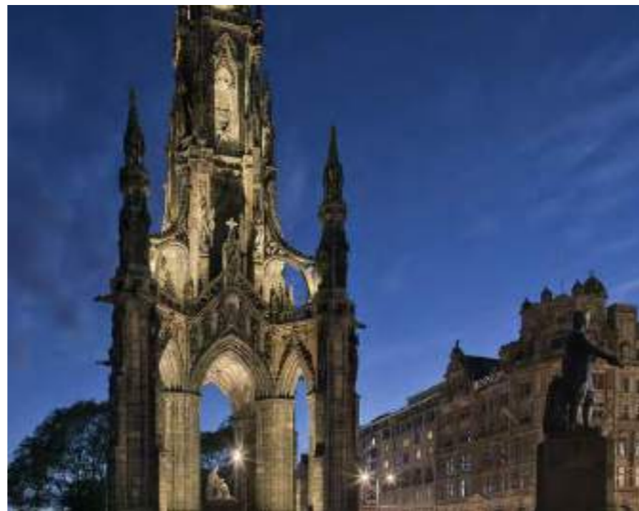
Use of accent lighting should be carefully planned to avoid over-illuminating all architectural elements and implement a visual hierarchy. A good example can be found in the Scott Monument Scheme. A subtle lighting approach in line with the surrounding context, revealing its architectural features in contrast.
